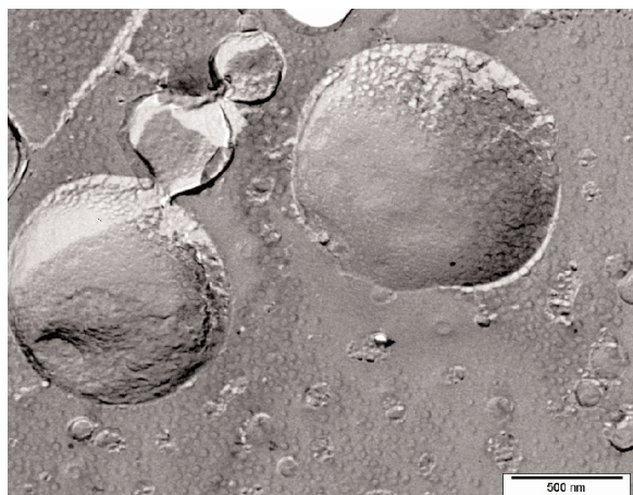
Figure 10: Cryo-TEM photograph of a O/W emulsion showing the bimodal droplet size distribution: 73.9 % wt water, 5 % wt Cremophor, mixture, 1.1 % wt paraffin oil.
