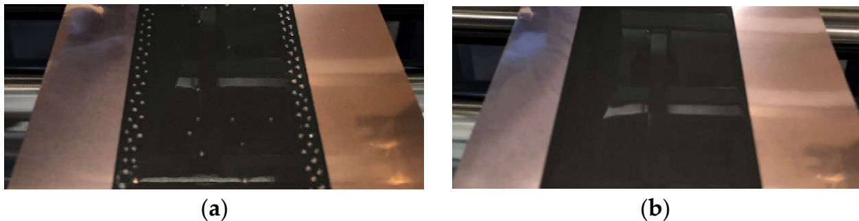
Figure 4. Inline photographs of the roll-to-roll coating experiments, web's direction from bottom to top; (a) coating outside stable operating window with visible air entrainment; (b) coating within the stable operating window.
