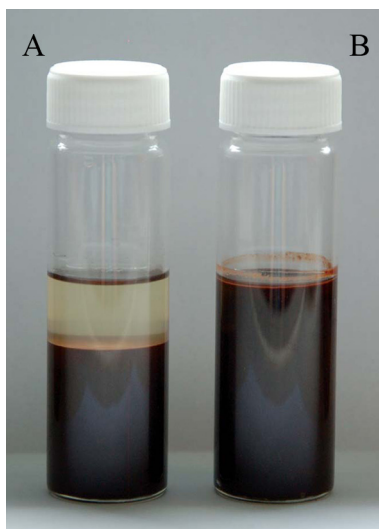
Fig. 3. Cocoa particles in oil \phi = 0.35 after a storage time of 5 days, (A) no water added, (B) water added (saturation S = 0.90 ).
